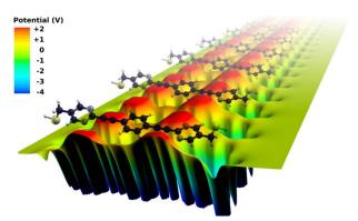
The collective electrostatic action of dipolar bonds at both ends of the molecules raises the electrostatic potential in the center of the monolayer (red region). Thereby, the quantummechanical states through which current can flow are lifted up in energy to more favorably align with those of external metal electrodes.
